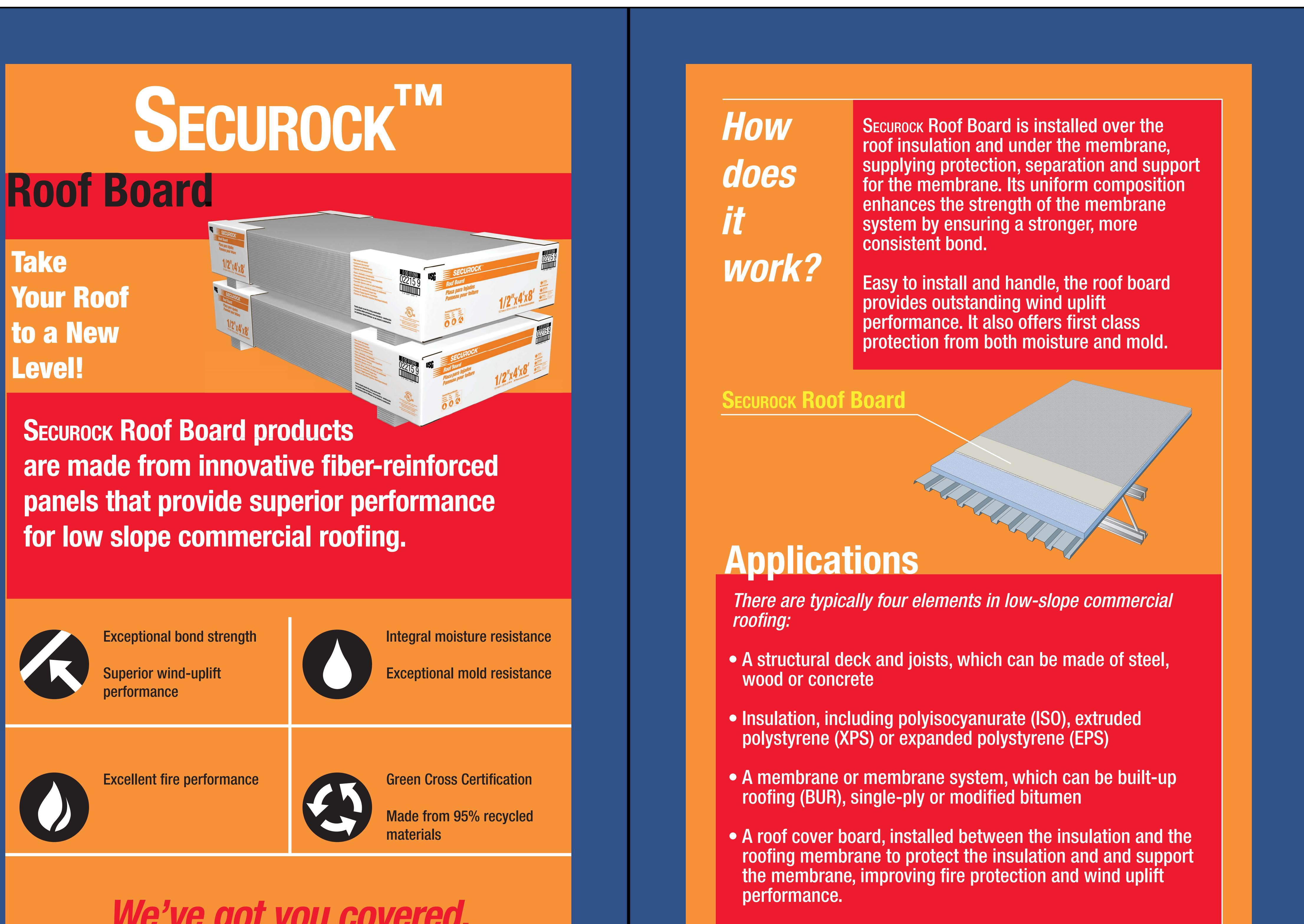
SECUROCK Roof Board products for low slope commercial roofing.
